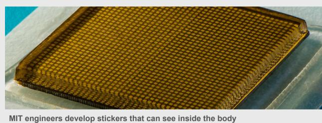
MIT engineers designed an adhesive patch that produces ultrasound images of the body. The stamp-sized device sticks to skin and can provide continuous ultrasound imaging of internal organs for 48 hours.
